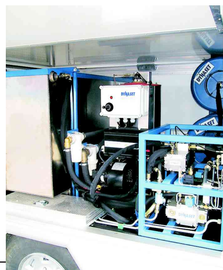
WHU water heater along with other DYNASET high pressure equipment installed to mobile pipe cleaner.
