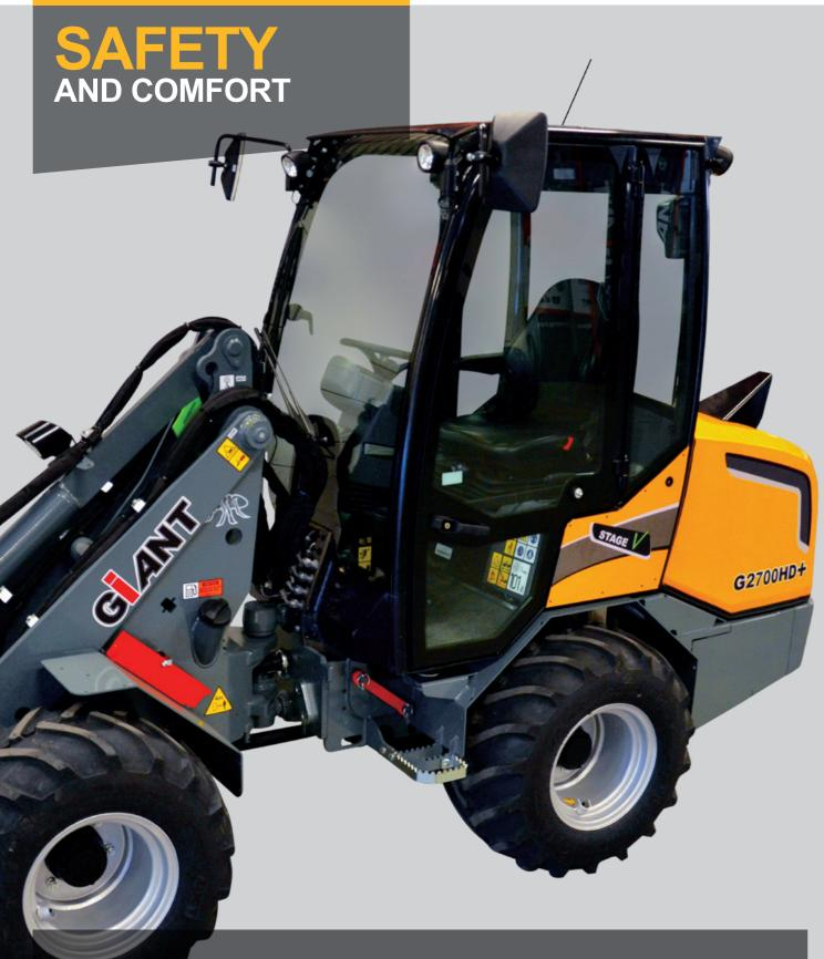
In the cabin, a comfortable working environment has been created so long working days are no problem. The steering column is fully adjustable and all necessary information can easily be read from a central display. While using the joystick, the operator can rest his arm on an ergonomically shaped armrest. All key functions are close to the joystick so that they can be operated without effort. Optionally, the machines can be supplied with items that are desirable for the work to be performed.
