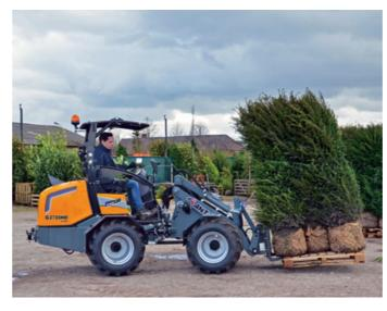
The powerful G2700 models are designed to operate in small spaces and on rough terrain. Not only the low weight and the compact dimensions ensure this, but also the articulated pendulum joint gives the machines a small turning circle and makes them extremely maneuvrable. This ensures that work can be done very accurately.
