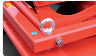
Four attachment points for safe transport
