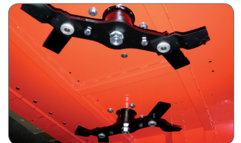
Deck design with custom designed blade carriers. Each carrier is equipped with four swinging blades offering breakaway protection in the event of impacts
