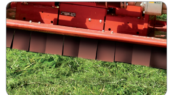
Heavy steel safety flaps reduce the risk of thrown objects
