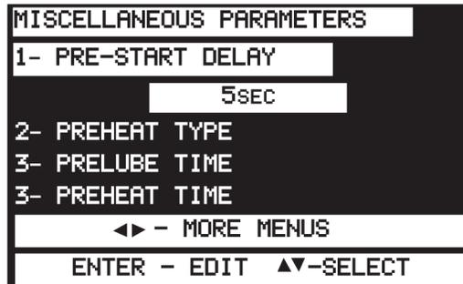
1. **Pre-Autostart Delay** - When system is in automatic mode, sets how long unit waits after a remote run signal is active before proceeding with automatic start sequence. (Default 5 seconds, set to zero to bypass.)
