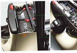
**Multiple battery options:** a variety of battery options are available including maintenance-free battery packs up to 192 Ah and industrial wet cell batteries up to 180 Ah (shown with optional central watering system).
