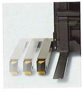
Adjustable outriggers: allows infinite adjustment of the outriggers from 865 - 1270 mm to provide for changes in storage and stacking requirements. Standard on ST and SX.
