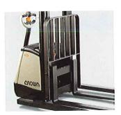
Load backrest: helps stabilise unsteady loads when travelling, lifting and lowering.
