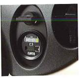
Battery discharge indicator: includes lift-lock-out and integrated hour metre.
