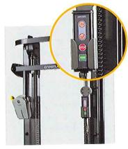
Remote raise/lower control: allows operator to control lift or lower function when using the stacker as a work positioner.
