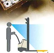
The sloped, low-profile power unit and clear mast design of the Crown Stacker Series provide excellent fork tip visibility (typically 50 percent of the total fork length).
