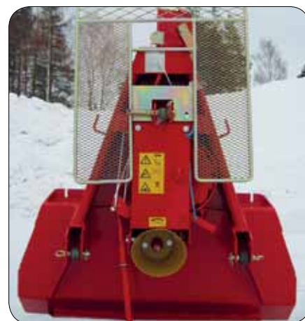
Power shaft in the center line of the winch
