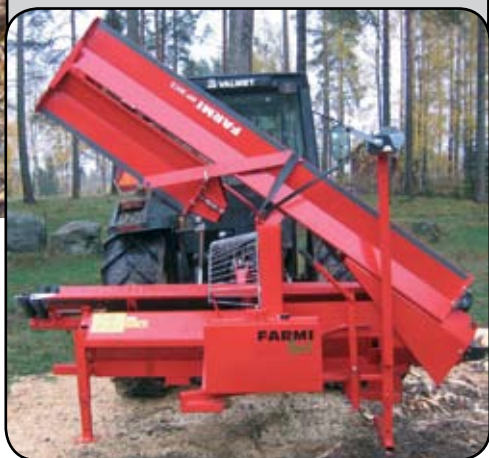
When in its transport position, the conveyor is locked over the machine.
