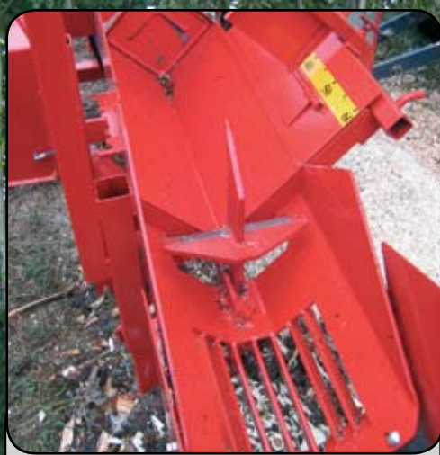
Debris and splinters fall down through the grating.
