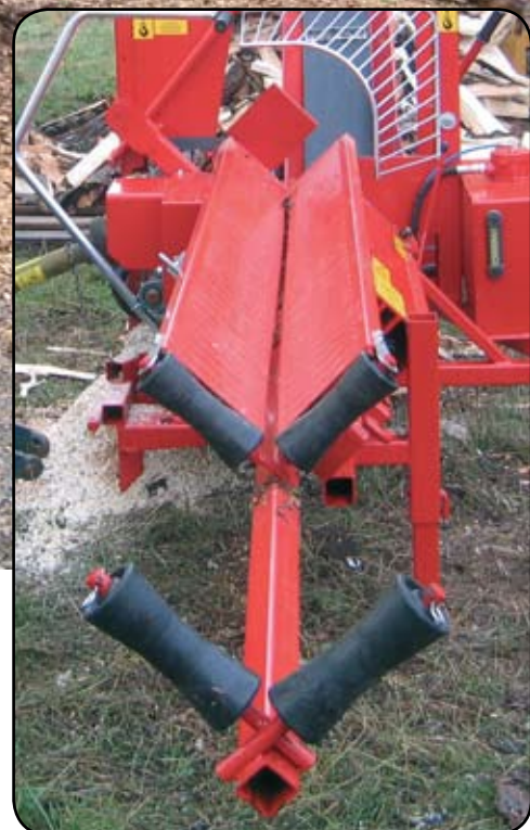
FARMI Mastersplit WP 30CS's unique patented feeding platform makes the job easier and faster. You simply operate the cross-cutting lever and the stem moves along on the feeding platform.
