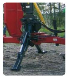
Primero's hydraulic stabiliser legs descend outwards, providing a stable platform to work even from side. Width of these Flap Down model legs (top to top as open is 3200 mm). Primero loaders can also be mounted to the tractor three point linkage.
