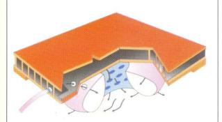
The GAPMASTER<sup>TM</sup> Aero-Caster® design includes a perforated membrane which meters the rate of air flow, resulting in the ability to cross gaps and steps.
