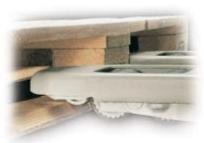
The exit ramp, riser and the exit roller are engineered for long life and impact resistance. The combined effect for the operator is excellent entry and exit from pallets, even when the pallet is empty. A low 75 mm lowered fork height allows easy access to difficult or damaged pallets.
